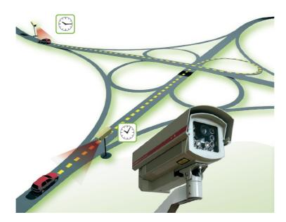
Smartspector's next generation traffic detectors facilitate a precise consolidation of passage data across locations. Digital signatures associated with individual vehicles allow for a reliable determination of comprehensive realtime travel time information.
